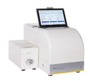
computer-controlled system, the instrument can regulate and control the temperature, humidity and flow rate precisely, which guarantee the testing sensitivity and repeatability of test results. C390H is applicable to determination of water vapor permeability of plastic films, sheeting, paper, packages and other relative packaging materials in food, pharmaceutical, medical apparatus, consumer goods, photovoltaic and electronic industries, etc.
